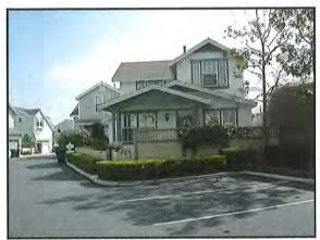
Use of a roof pitch 1:4, shown for entry) lower than that of the main building (1:3, shown for main roof) is considered acceptable.
